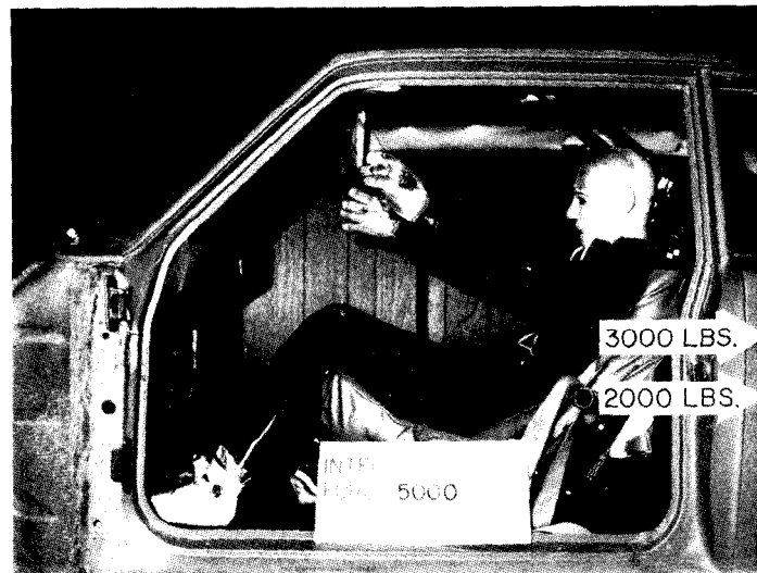
Fig. 8 - Integrated seat during testing; 2268 kg (5000 lb) force applied rearward
