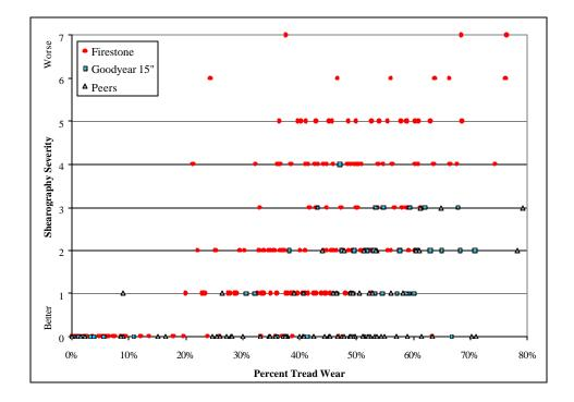
Figure 21 – ODI shearography analysis comparing Firestone focus tires and their Goodyear and non-Goodyear peers by belt edge separation severity. Separation categories are defined in Appendix A
