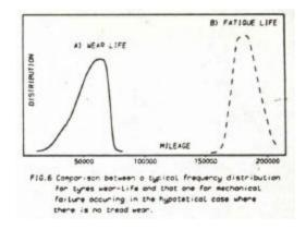
"Curve A represents the frequency distribution for the tyre's wear life in its various uses. Curve B represents product life distribution for mechanical failure occurring in the hypothetical case where there is no tread wear.
