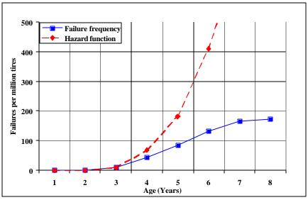
Figure 17 – Comparison of cumulative hazard function vs. cumulative failure frequency, Wilson ATX P235/75R15 tires. Firestone claims database as of March 2001
