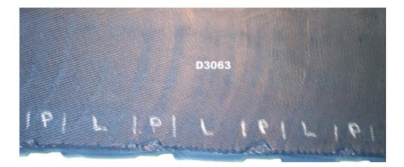
Figure 31 – Localized separation pattern on tread pull of the same tire; "P" = pocket area, "L" = lug area.
