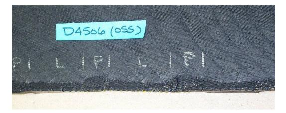
Figure 33 – Belt-edge separation pattern showing growth in pocket areas of the same tire; "P" = pocket area, "L" = lug area.
