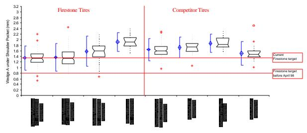
Figure 36 – Wedge gauge under shoulder pocket, Focus tires (after the 1998 design change) vs peers.
