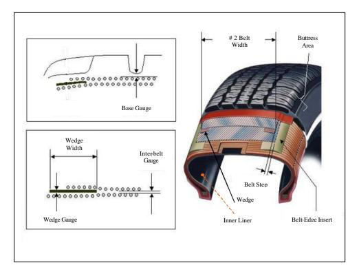
Figure 7 – Radial tire construction.
