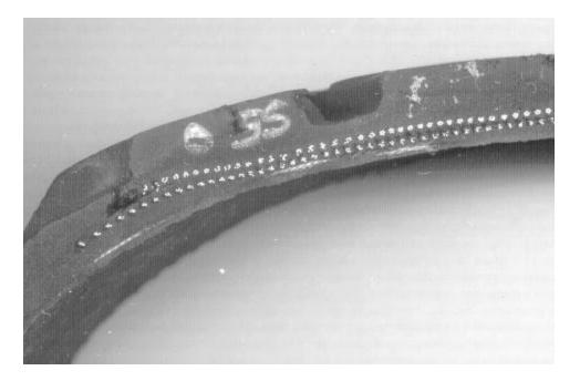
Figure 20 – Wilderness AT pocket crack growth to edge of No. 2 belt Wilson P235/75R15 Wilderness AT tire, manufactured in Oct 97 (W2 417).
