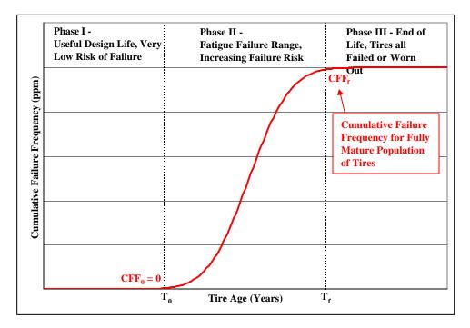
Figure 12 – Fatigue failure theoretical model.
