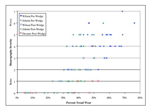
Figure 23 – ODI shearography analysis comparing P255/70R16 pre- and post-wedge change focus tires by belt edge separation severity. Separation categories are defined in Appendix A
