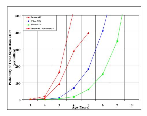
Figure 18 – Cumulative hazard function, recalled tires, by model and plant. Firestone claims database as of March 2001
