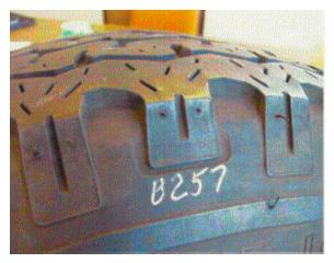
Figure 1 - Ford-Spec P235/75R15 ATX
