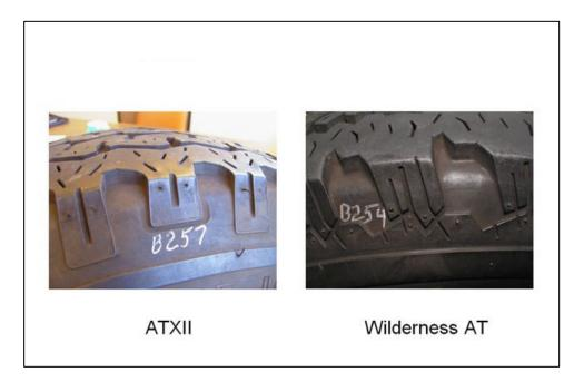
Figure 8 – Shoulder pockets in ATX and Wilderness AT P235/75R15 Tires manufactured for Ford.
