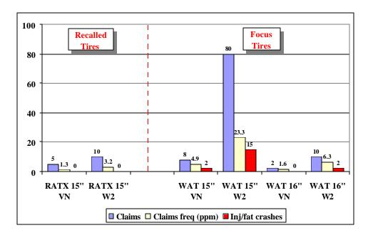
Figure 15 – ATX vs. Wilderness AT, failure experience comparison, by plant; 56 months after first tire produced.
