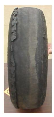
Figure 10 – Separation pattern on the tire carcass of a failed Wilson P235/75R15 Wilderness AT tire, manufactured in Sep 96 (W2 396).
