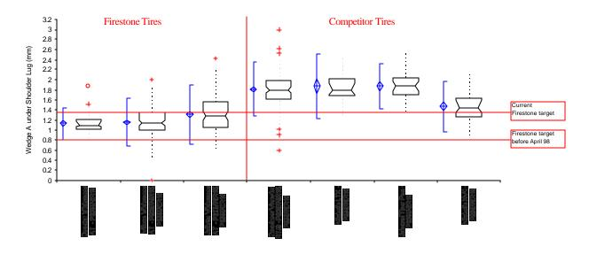
Figure 25 – Wedge gauge under shoulder lugs, Focus tires (prior to 1998 design change) vs. peers.
