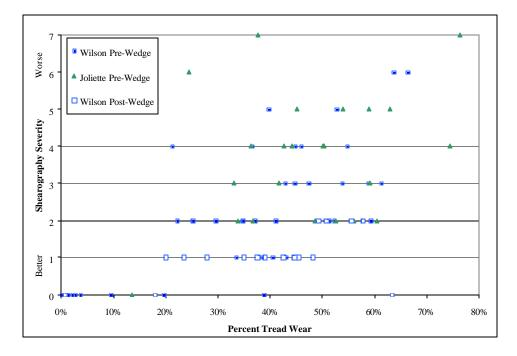
Figure 22 – ODI shearography analysis comparing P235/75R15 pre- and post-wedge change focus tires by belt edge separation severity. Separation categories are defined in Appendix A
