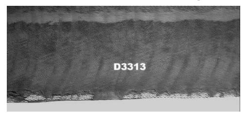
Figure 38 – Tread-pull from test program tire with belt edge separation; Wilson P255/70R16 Wilderness AT tire, manufactured Jun 97.
