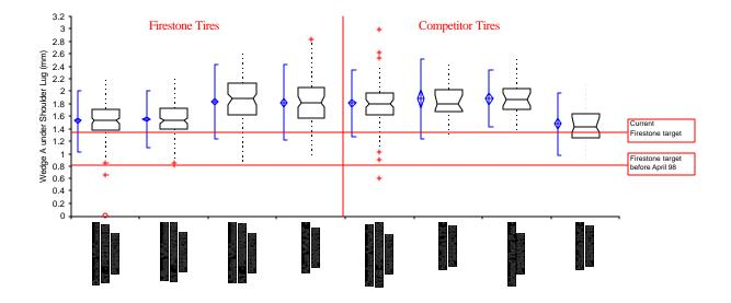
Figure 26 – Wedge gauge under shoulder lugs, Focus tires (after 1998 design change) vs. peers.
