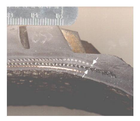
Figure 34 – Wedge "pinching" under shoulder pocket, Wilson P255/70R16 Wilderness AT tire, manufactured in Nov 97 (W2 487).
