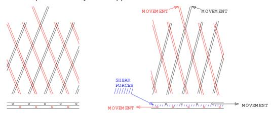
Between the belts is a layer of rubber usually referred to as the interbelt rubber. The opposing radial movement of the steel belts causes the interbelt rubber to be distorted because the interbelt rubber attached to the top belt is pulled in the opposite direction to the interbelt rubber attached to the bottom belt.
