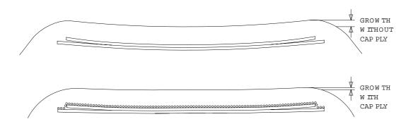
The physical restriction of the cap ply causes the movement of the belt edge to be significantly reduced and this has three very important and significant consequences:
