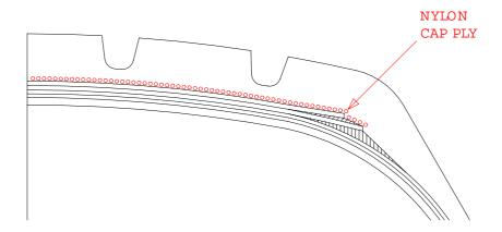
The cap ply is a mechanical device that acts a kind of tourniquet and restricts the amount of growth due to the centrifugal load on the tire:
