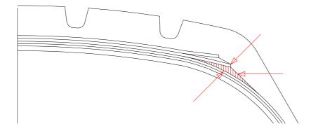
The shoulder insert acts as a cushion between the ply and the belt so it absorbs a lot of mechanical energy, some of which is converted to heat energy. For this reason it is important that the insert compound is formulated so that it retains as little heat as possible or, as it is known in the tire industry, it is a "cool running" compound.
