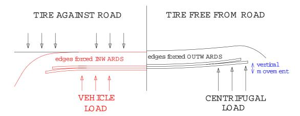
The diagram shows that there is considerable movement at the belt edges during this cycle and this considerably increases the stresses around the belt edges.
