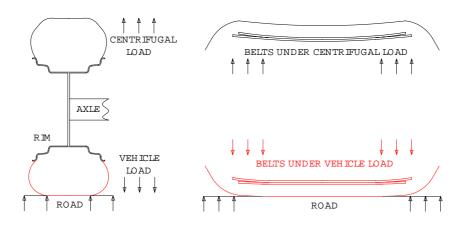
As it continues to rotate the small section passes out of contact with the road and is subject to the load exerted by the centrifugal force generated by its rotation.
