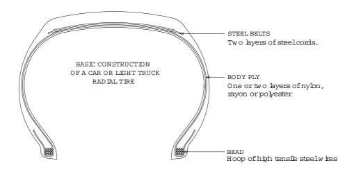
This diagram shows the steel and textile reinforcements, the skeleton, of a radial tire.
