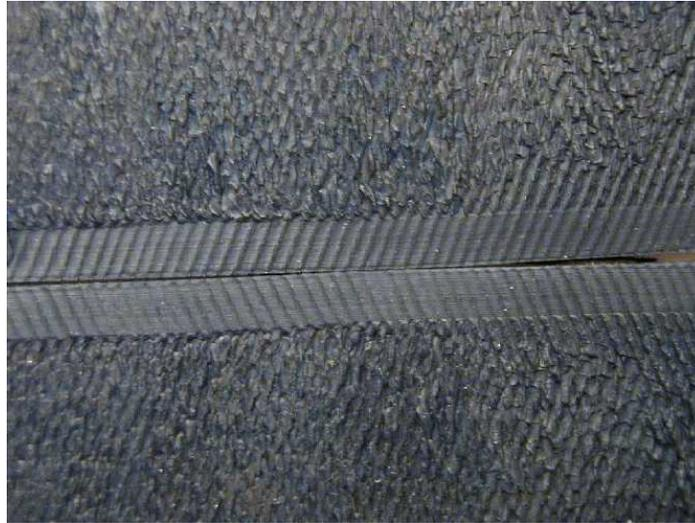
Figure 21: Peel test surface for F89 manufactured in Wilson. Distance between reflective peaks of steel cords is approximately 1.4 mm.
