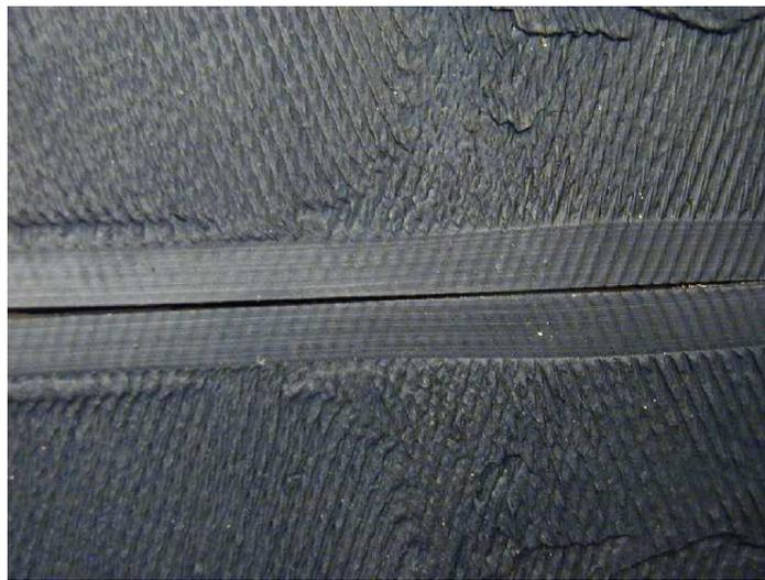
Figure 20: Peel test surface for F44 manufactured in Decatur. Distance between reflective peaks of steel cords is approximately 1.4 mm.
