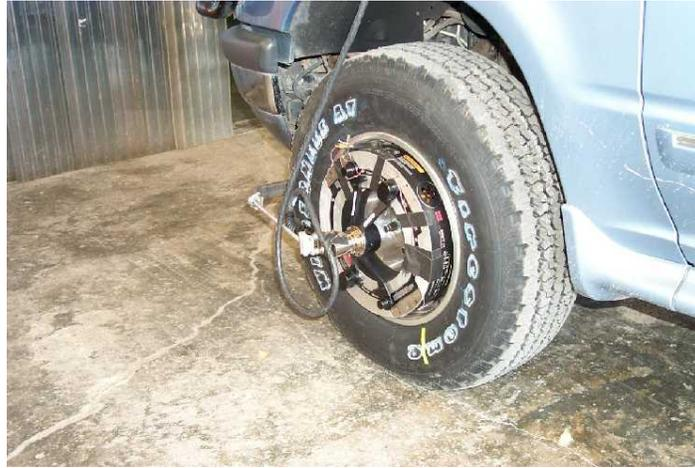
Figure 6: Close-up view of load cell affixed to tire.
