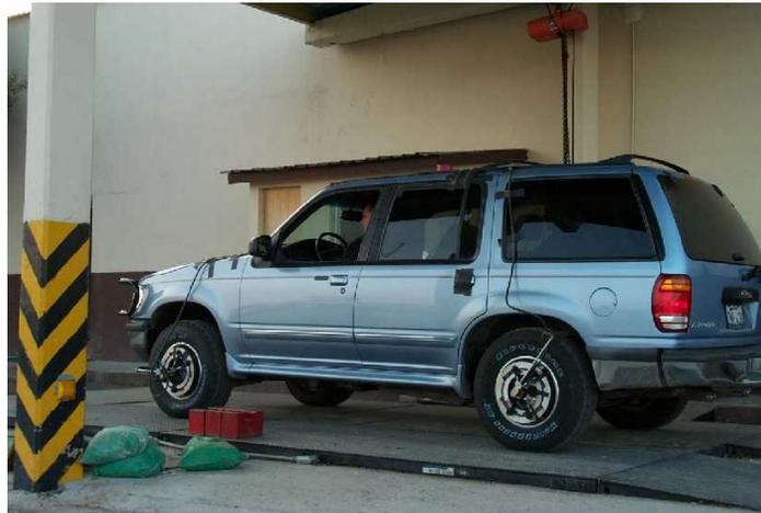
Figure 7: Side view of Ford Explorer with load cells attached.
