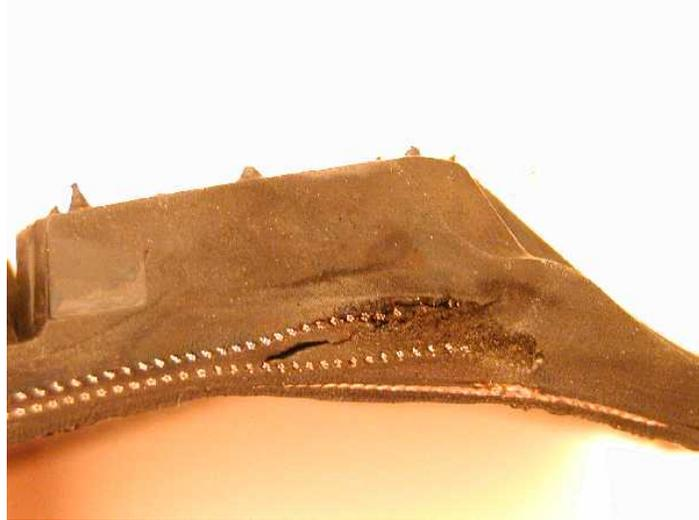
Figure 1: Belt edge crack example from a steel belted radial tire.
